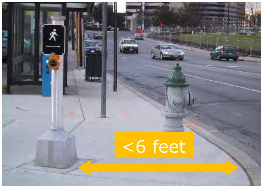
Figure 7 – Pushbutton relative to curb face
